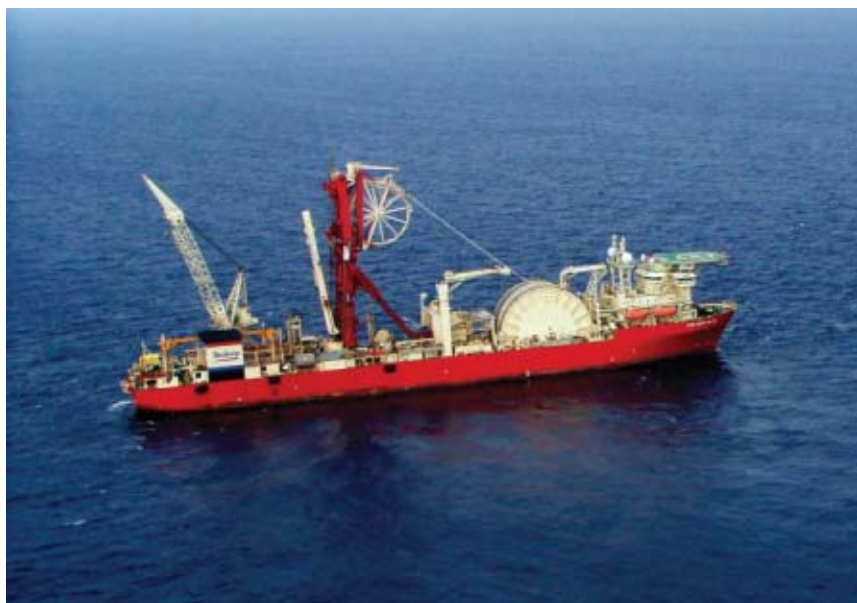
Technip Deep Blue will install the dual 10 inch ANF flowlines in 2008.
