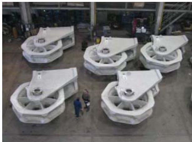
Seven Pocket Fairleader for 171 millimeter Chain
