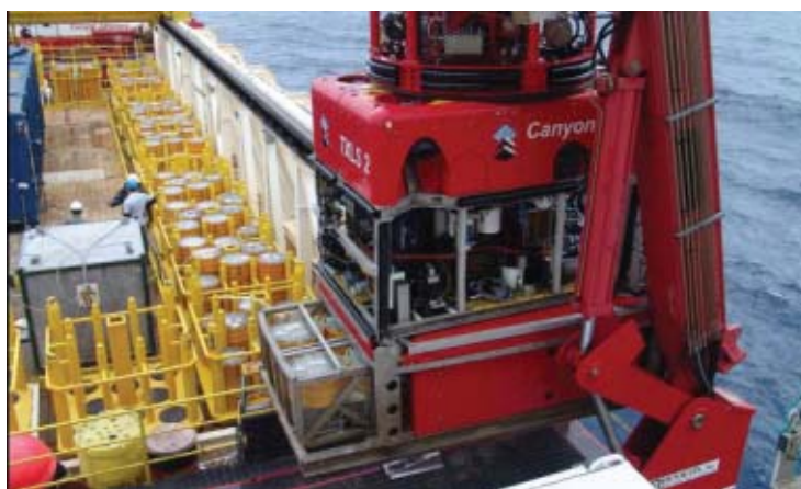
ROV loaded with OBS nodes ready to deploy to the seafloor
