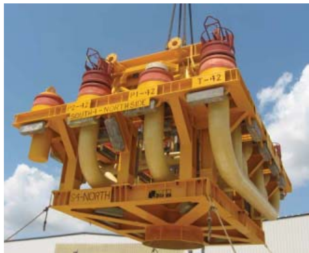
Manifold fabricated and tested at Oil States Houston
