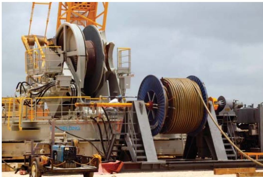
Spooling Winch Wire at Ingleside, TX
