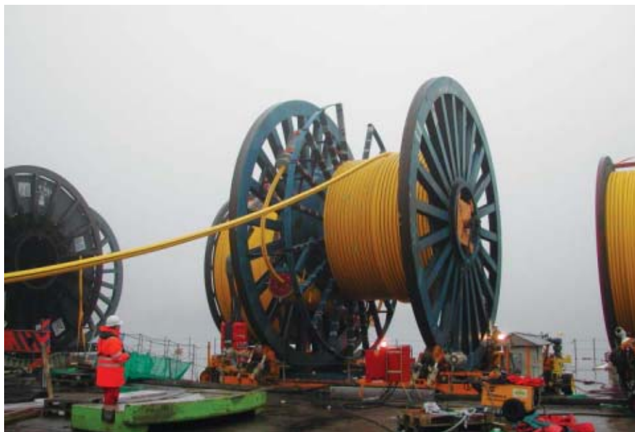
Atlantis umbilicals being spooled to reels before shipment to Gulf of Mexico.
