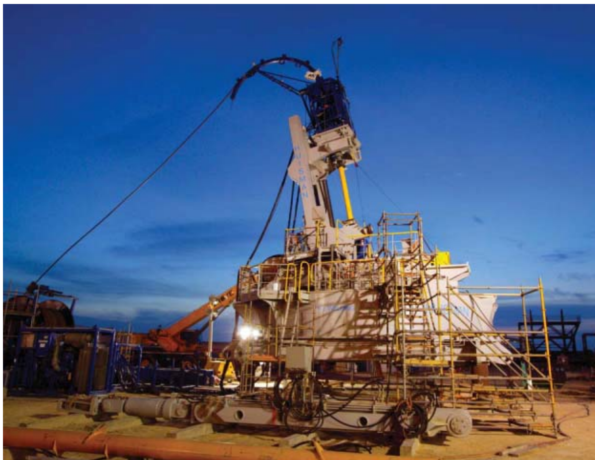
Coiled Tubing Unit Testing at Ingleside, TX
