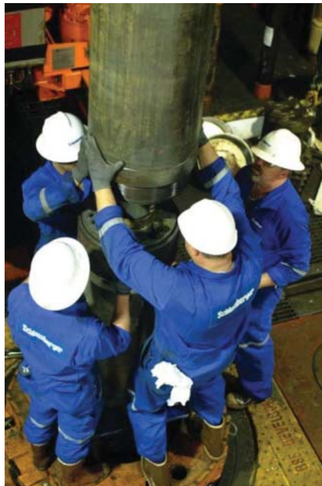
Schlumberger field technicians supervise the deployment of the Sen-TREE 7 test tree and Commander control system used for completion installation and subsea latching/unlatching of the landing string to subsea completion.
