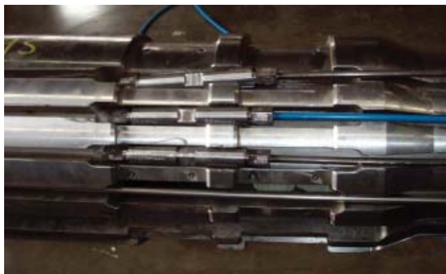
Baker Oil Tools used a milled sleeve to house and protect the Intelligent Well System control line splices.
