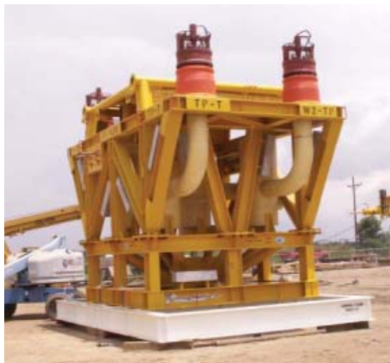
One of multiple PLEMs built for BP Atlantis DC1 project.
